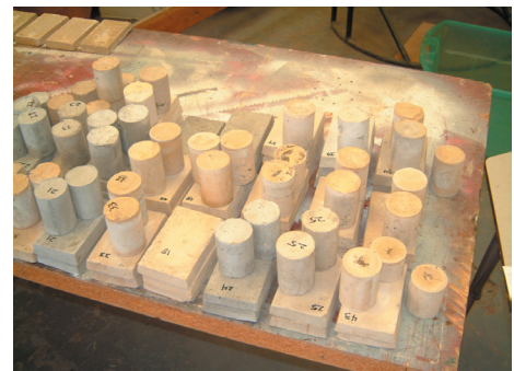
Cylinders and slabs made using flyash as the primary cementitious binder, along with a variety of aggregates.
